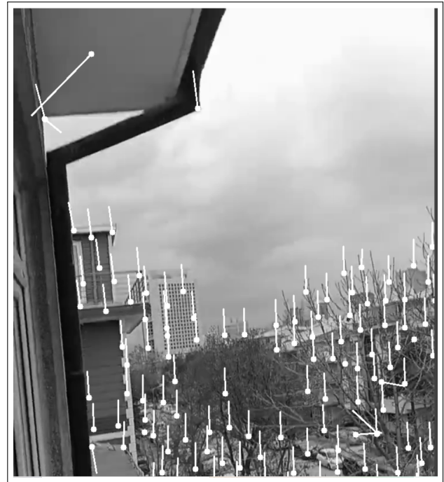
Fig. 3. The calculated optical flow of feature points.
